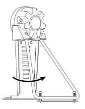
Use a tuning key supplied with the FD-8 to tighten the screws removed in Step 1 so that the stand is firmly secured.
